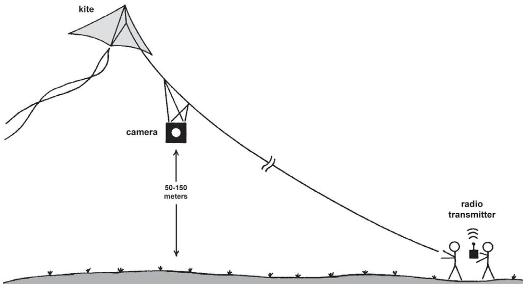
Figure 1. Cartoon showing setup for kite aerial photography (KAP). A radio transmitter on the ground controls operation of the camera rig. Illustration not to scale. Adapted from Aber, Zupancic and Aber (2003, fig. 1).
