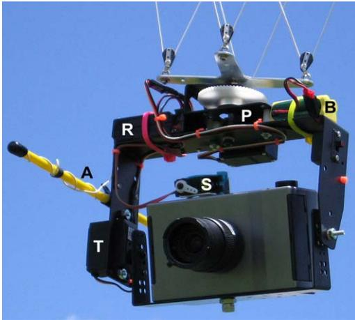
Figure 3. Radio-controlled rig for kite aerial photography with the Tetracam ADC digital, color-infrared camera. R - radio receiver, P - pan servo and gears, B - NiMH battery pack, A - antenna mast, S - shutter miniservo, and T - tilt servo.
